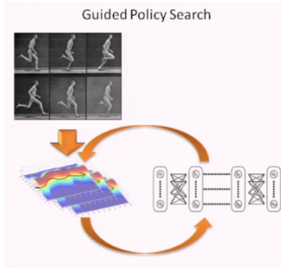
Figure 2.10: GPS operating diagram: on the left is the “instructor” algorithm, generating trajectories, that feeds the neural network on the right (from Levine et al. (2015b,a) ; Levine and Abbeel (2014) )
